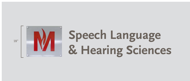
Vinyl Verbage - 6"- 8"h, 1/16" Brushed Aluminum Back - 18" x 18", 4 Aluminum Stand-offs, 3-D Acrylic Logo, DS Tape Mount
