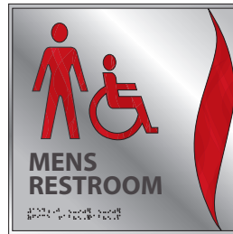
10" x 10" Restroom - Men • Insert with Aluminum Frame 1/16" 2-ply & 1/32" Brushed Aluminum/Black (Back Plate) 1 MM Sintra White (with Digital Print) 1/16" 2-ply & 1/32" Brushed Aluminum/Black with Charcoal Gray Verbage Braille: American
