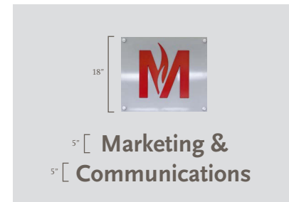
Vinyl Verbage - 5"h, 1/16" Brushed Aluminum Back - 18" x 18", 4 Aluminum Stand-offs, 3-D Acrylic Logo, DS Tape Mount
