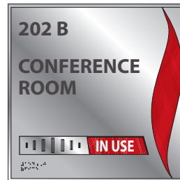
10" x 10" Conference Room with Slider • Insert with Aluminum Frame 1/16" 2-ply & 1/32" Brushed Aluminum/Black (Back Plate) 1 MM Sintra White (with Digital Print) 1/16" 2-ply & 1/32" Brushed Aluminum/Black with Charcoal Gray Verbage Braille: American
